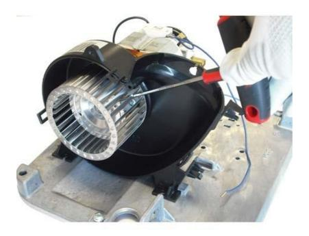
Remove the fan from the drive shaft.
