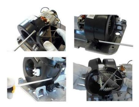
Remove the heating element for replacement.
