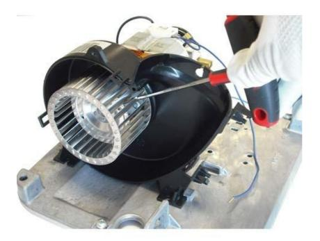
Remove the fan from its position and replace it.
