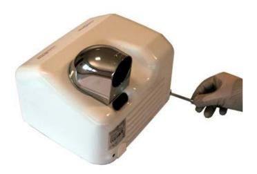
Carefully remove the casing.
