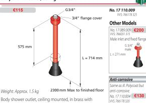
Body shower outlet, ceiling mounted, in brass with chemical resistant BROEN Polycoat with self-draining shower head. Fits different ceiling heights by adjusting the flange. Inlet G 3/4" male.
